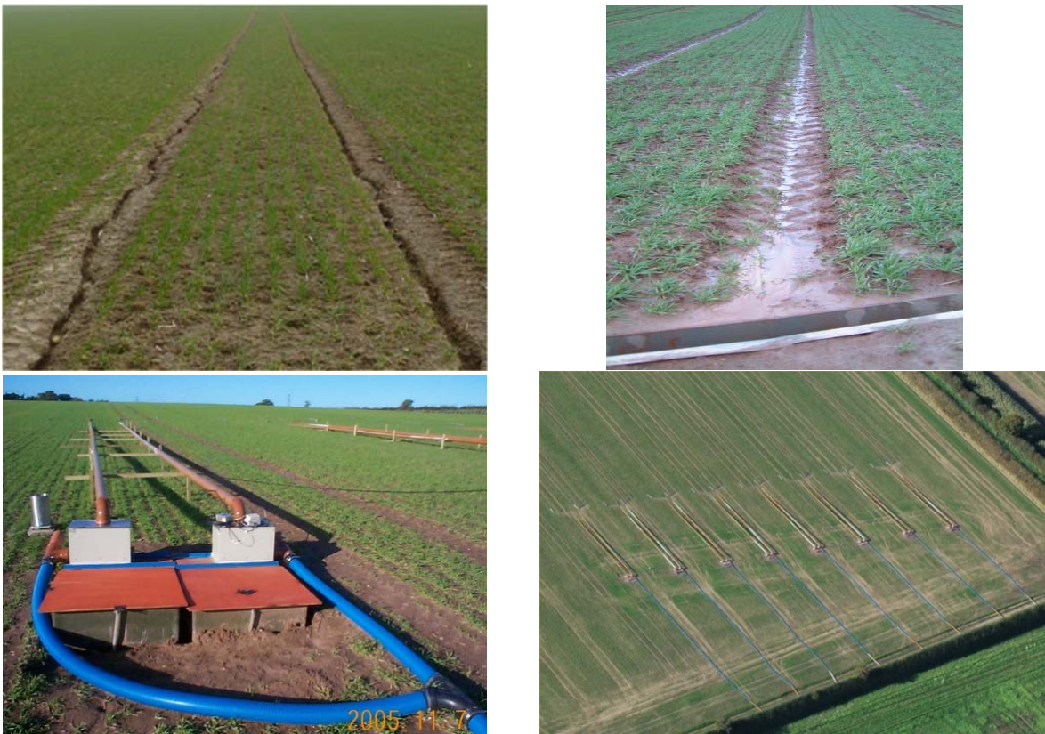
Figure 7. Rills in tramline wheelings at silty clay loam site following autumn spraying (top left); gutter collecting runoff from tramline wheeling during rainfall event at loamy sand site (top right); monitoring equipment in situ on two adjacent plots with orange pipework, white sample splitters, black runoff collection tanks with red lids, and blue wastepipes (bottom left); and aerial view of 16 plot experiment monitoring tramline treatments (bottom right).
