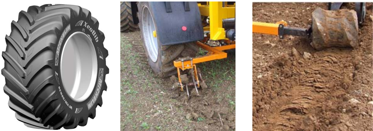
Figure 1. Experimental treatments: VF tyre (left), rotary harrow (middle), and surface profiler (right)
