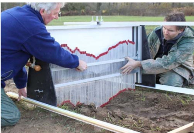
Figure 9. ADAS staff taking soil surface roughness measurements using the bespoke pin meter unit. The horizontal bar at the top of the unit was attached to a digital camera (out of shot), which recorded the height of individual pins across the tramline.
