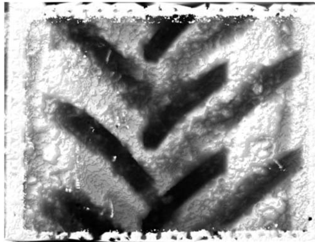
Figure 20. Example DTM developed for the Hattons CT wheeling in 2010 using Erdas eATE. The cleat impressions are darkest, representing approximately 0.06m depth from the soil surface. The field of view is 0.8m.
